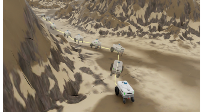
Fig. 9: Smooth and continuous trajectory generation based on traversability maps in the Isaac Sim
